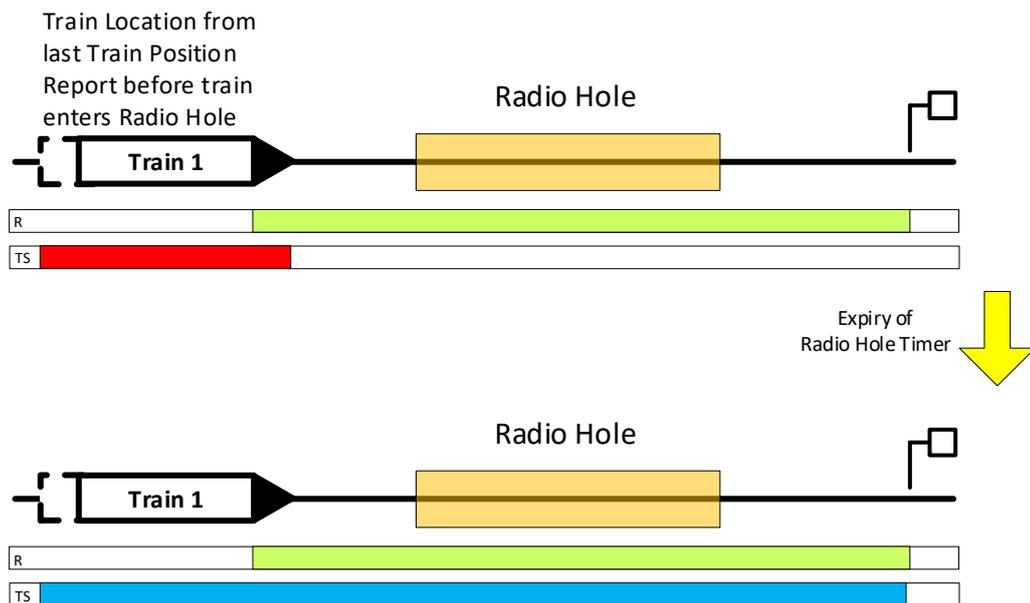
**Figure 42: Unknown area after expiry of Radio Hole Timer**
