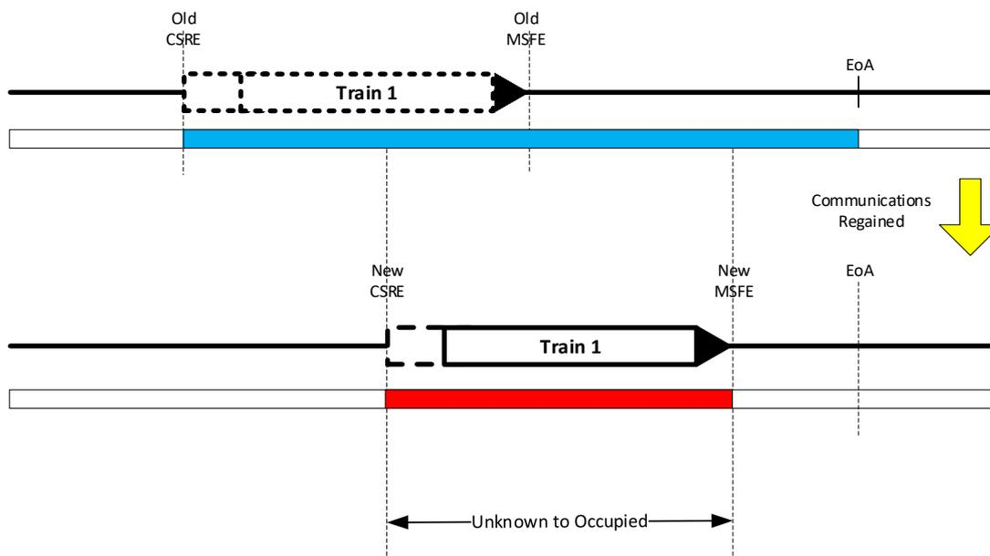
**Figure 41: Unknown to Occupied Transition following reconnection of communications**
