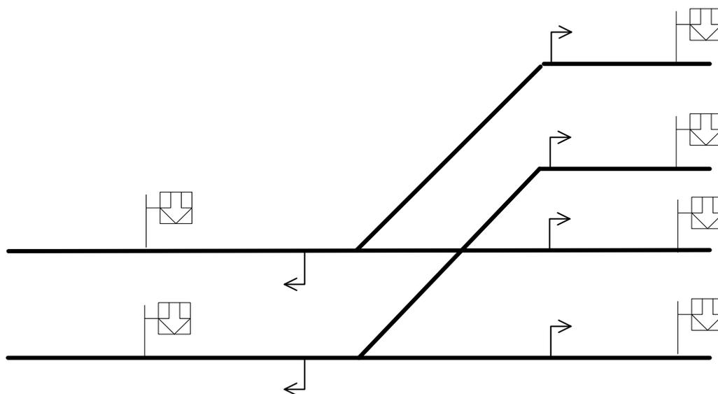
**Figure 31: Release Points at a double junction**
