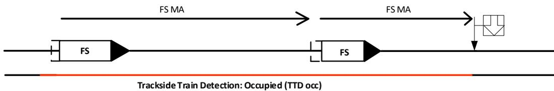
Figure 6 – Overview System Type Full Moving Block with Trackside Train Detection
