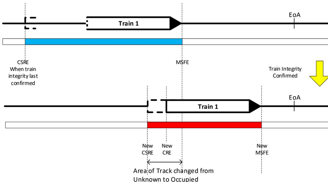
**Figure 45: Unknown to Occupied Transition following regaining train integrity**
