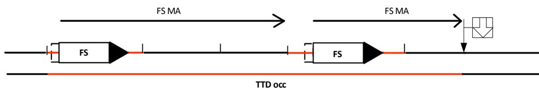
**Figure 8 – Overview System Type Fixed Virtual Blocks with Trackside Train Detection**
