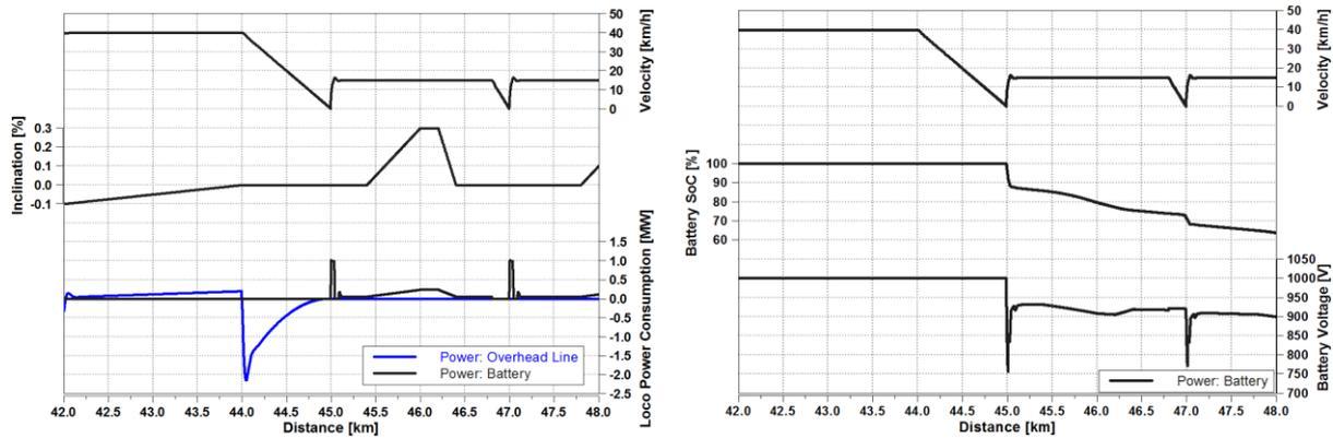
Fig. 3 Simulation results, (a): track profile & power consumption, (b): battery SoC & voltage.
