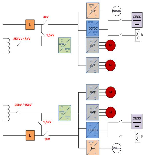
Fig. 1 Simplified one-line diagram of a Hybrid Electric Multi-System locomotive
