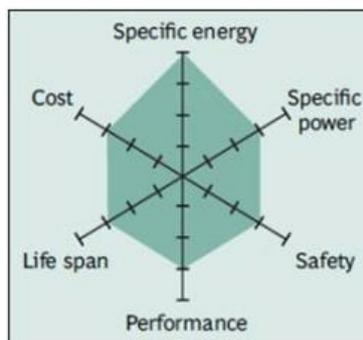
Figure 4: nNMC characteristics, Courtesy of Cadex
