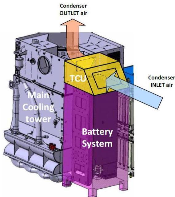
Figure 5: Battery cubicle with air flow of the TCU
