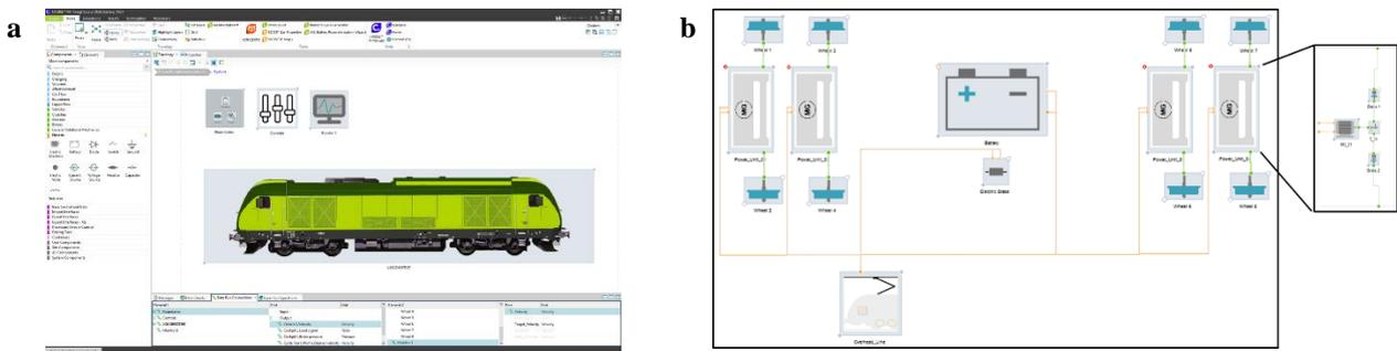
Fig. 2 (a) (b) Simulation model overview of a BoBo Hybrid Electric Multi-System locomotive on CRUISE M.
